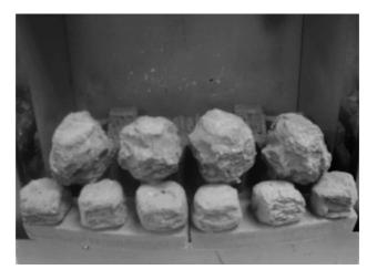
e) Select three of the small coals and fit onto the ribs of the fuel-bed base. See fig. 5 below
